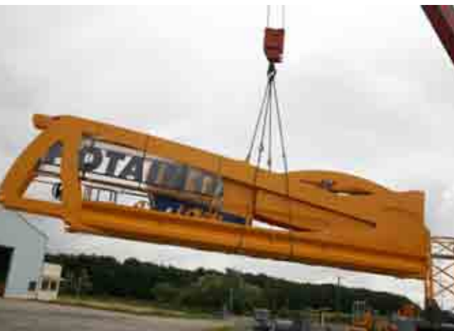
Compact counter jib with nose and wind-sail plate, designed to be folded up during transportation.
