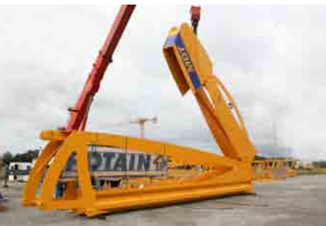
Simple unfolding of counter-jib nose and wind-sail plate frees the grab rails.
