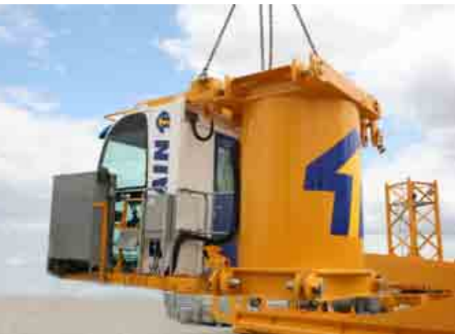
Cab/mast-cab in a single compact package.
